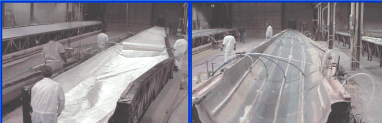
TPI manufactures wind turbine blades in Warren, RI
